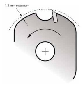
Figure 2 An example of a non-round form tool with limited cutter projection
