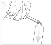
Use shadow vacuuming to control dust as you remove screws
