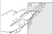
If possible, remove nails with a claw and shadow vacuuming. If this is difficult without damaging the board, apply paste to one corner and make a deep score line so you can lever the corner away first
